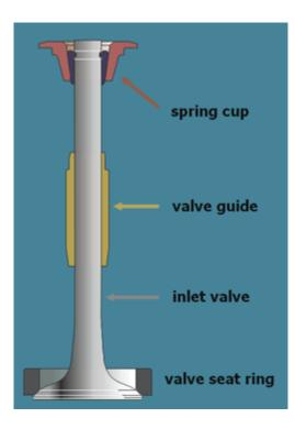
Fig. 5 Inlet valve with possible Al parts (courtesy PLM)
