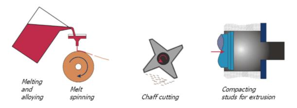
Fig. 2 Processing steps for high performance aluminium (courtesy PLM)
