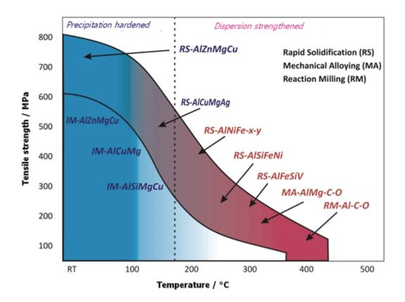
Fig. 1 Tensile strength versus temperature of aluminium alloys (courtesy PLM)
