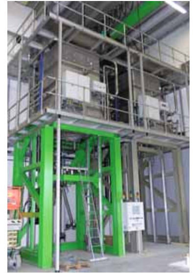
Fig. 6 Twin-furnace for series production of RSiC diesel particulate filters
