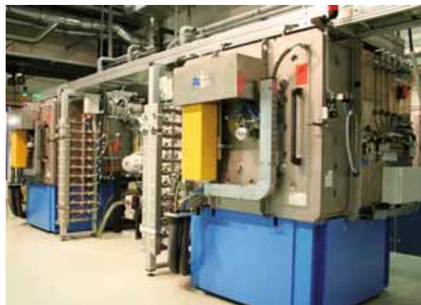
Fig. 4 Twin-furnace for pyrolyzing and silicizing C/SiC parts
