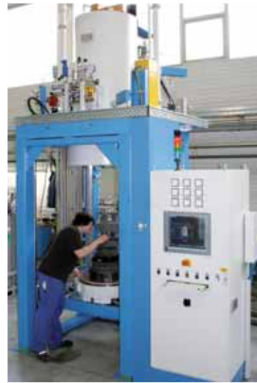
Fig. 8 Gas pressure sintering furnace for up to 100 bar at 2200 °C
