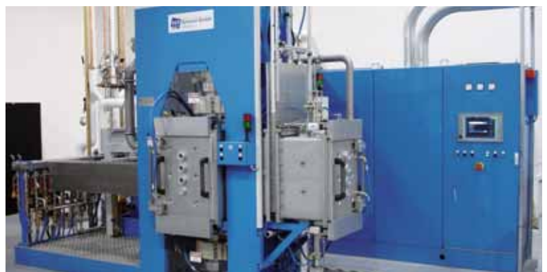
Fig. 11 Two-chamber FAST/SPS machine for highly efficient production of sputtering targets
